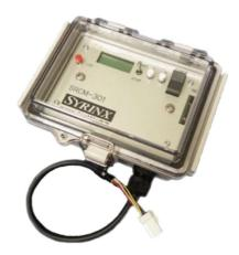
Since it is powered by a built-in battery, there is no need to secure an external power supply, making it possible to measure in a variety of environments. The one-touch connectors are used to connect the sensor cable and logger for easy connection. Because of its compatibility, it can be installed in narrow places.
